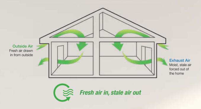
Positive Pressure Systems are ideal for managing moisture and humidity within your home. These systems draw in fresh air from the roof cavity and filter it before distributing the clean air around your home via a network of ceiling diffusers. The air movement forces the moist, stale air that causes condensation, mould and mildew out.
